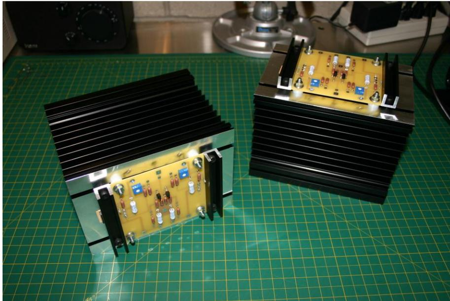
Once the channels are complete you'll need to attach them to the top plate with M5 hardware. Slide a hex head bolt into each T-slot on either side of the PCB then, lower the top plate over the heat sink assembly and align the bolts with the four mounting slots in the top plate. Center the heat sink and square it up with the top plate, then fasten with washers and M5 nuts as pictured below.
