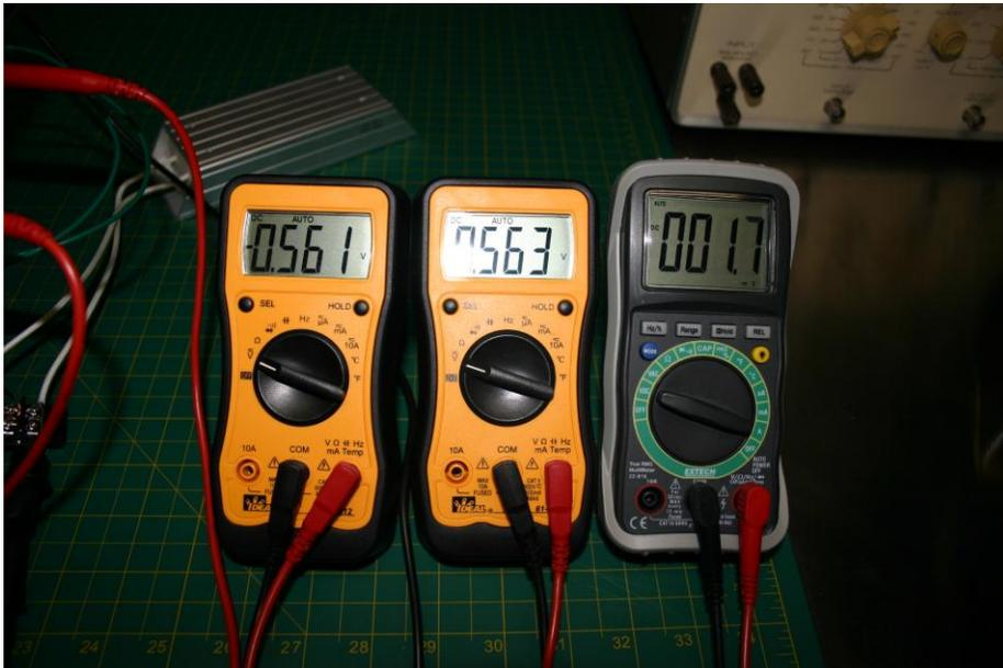
Here we are using three meters to dial everything in. Set the bias, and set it again after a few hours warm-up with the chassis box on. Once the bias is set, and reset, you can permanently attach the whole top plate assembly to the box with wood screws.
